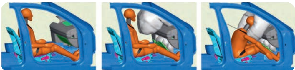
Figure 4.7 Airbag systems in vehicles are designed to deploy during vehicle collision
