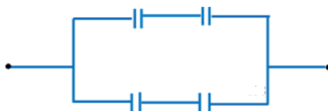
Figure 6.55: Reduced equivalent circuit of the network shown in Figure 6.54.
