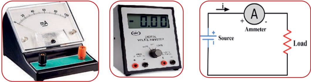
Figure 6.27: Ammeters and How to connect them.
