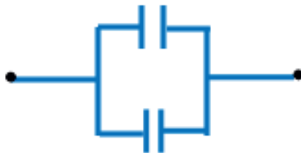
Figure 6.56: The equivalent capacitance of the network in Figure 6.54
